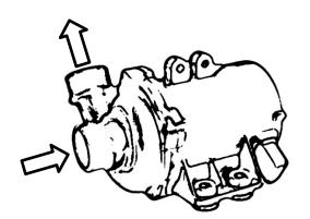
**Attention:** Please only mount the pump with appropriate rubber dampers because high vibration can damage the internal electronics!
