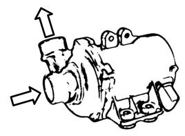
**Attention:** Please only mount the pump with appropriate rubber dampers because high vibration can damage the internal electronics!
