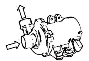
**Attention:** Please only mount the pump with appropriate rubber dampers because high vibration can damage the internal electronics!
